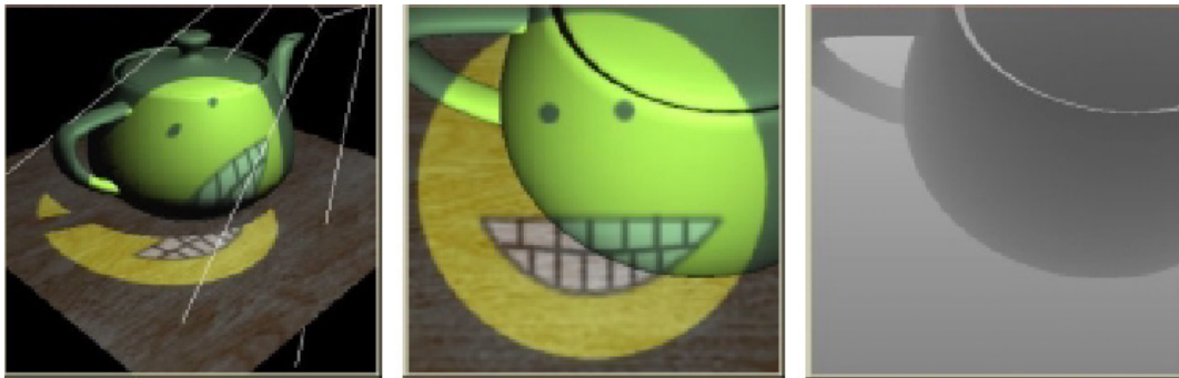
Figure 2: Shadow mapping in stages. Figure from Cebenoyan (2001).
